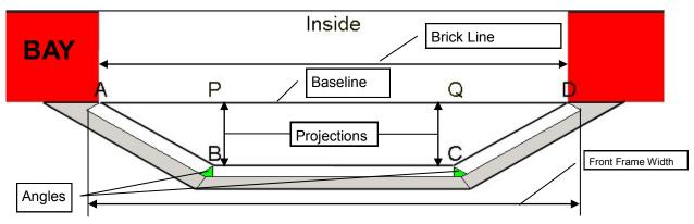
Bay information. To start measure the existing frames wooden or plastic. Measure the base line and the angles or the projection of the bay. We will do the rest.
