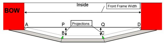
Bow information. To start Bow's are different than bays as originally there was no bay. These are know as bow bay conversions. The reason it's a conversion is usually there used to be a normal window in the hole and the customer wants a bow bay conversion. First you will need to measure the front frame width or Brick to Brick size and the projection which is measured from the reveal. The frames sizes are usually all the same size this only changes when static or variable bay poles are used.
