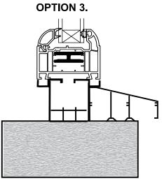
Fitted in the conventional way the upstand is only 52mm while conventional PVC-u Bi-Folding doors have an upstand between 100mm and 140mm
