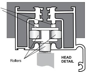
The HEAD & THRESHER are aluminium and do not have a PVC-u frame
